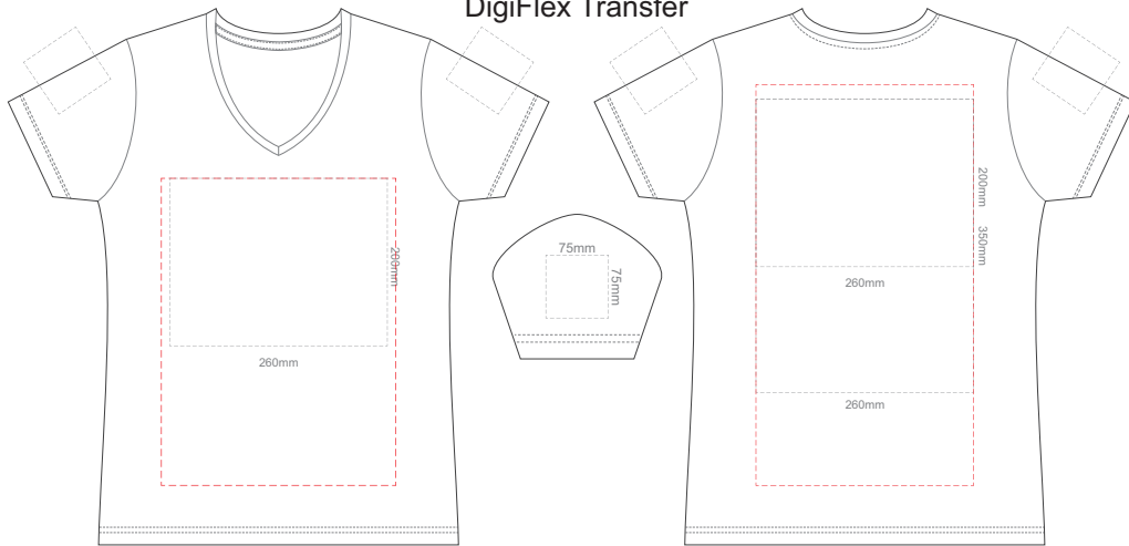
FRONT WOMEN'S MEDIUM Print area can be rotated to best suit. Branding area can be moved anywhere within the red line.
