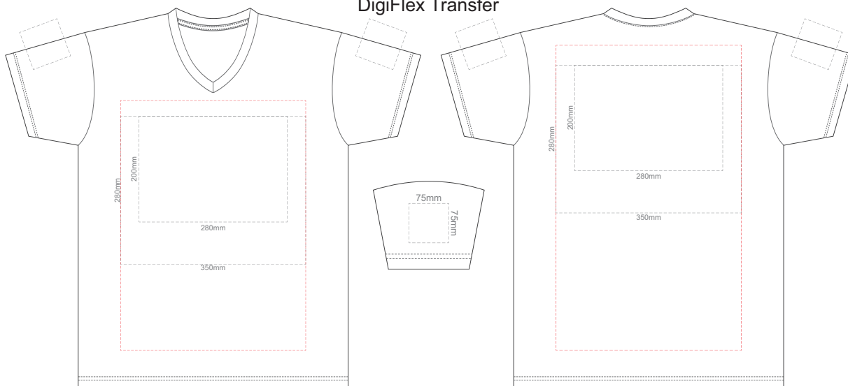
FRONT ADULT MEDIUM Print area can be rotated to best suit. Branding area can be moved anywhere within the red line.
